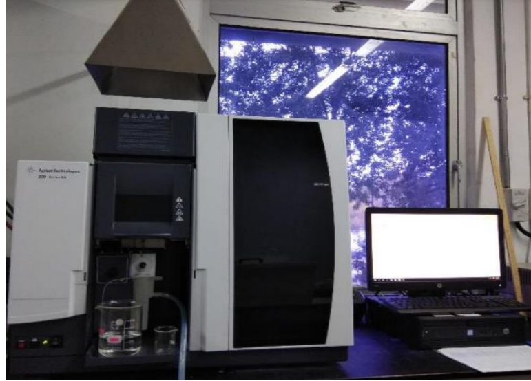
Figure 3.4: Single-beam flame atomic absorption spectrophotometer (FAAS)
