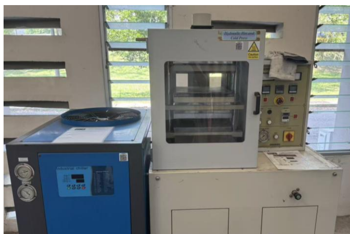
Figure 3.2: Hydraulic Moulding Press (GOTECH GT-7014-H, GOTECH Testing Machines Inc., Taiwan).
