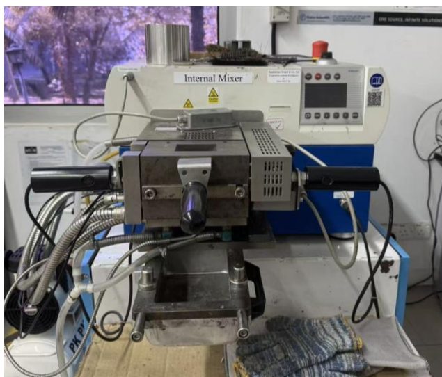
Figure 3.1: Brabender Internal Mixer (Plastograph EC 815652, Brabender GmbH & Co. KG, Germany).
