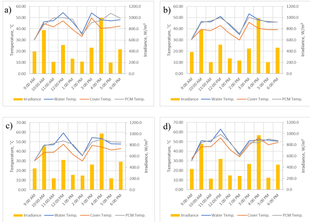
Figure 4.16: Temperature and irradiance results for different PCMs using 20k ppm saline water and FL 33 cm Fresnel lens (a) Al 2 O 3 and Cu NPCM (b) Al 2 O 3 NPCM (c) Al scrap PCM (d) Cu NPCM
