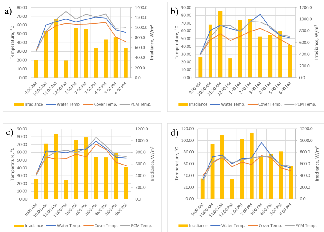
Figure 4.14: Temperature and irradiance results for different PCMs using 10k ppm saline water and FL 33 cm Fresnel lens (a) \text{Al}_2\text{O}_3 and Cu NPCM (b) \text{Al}_2\text{O}_3 NPCM (c) Al scrap PCM (d) Cu NPCM
