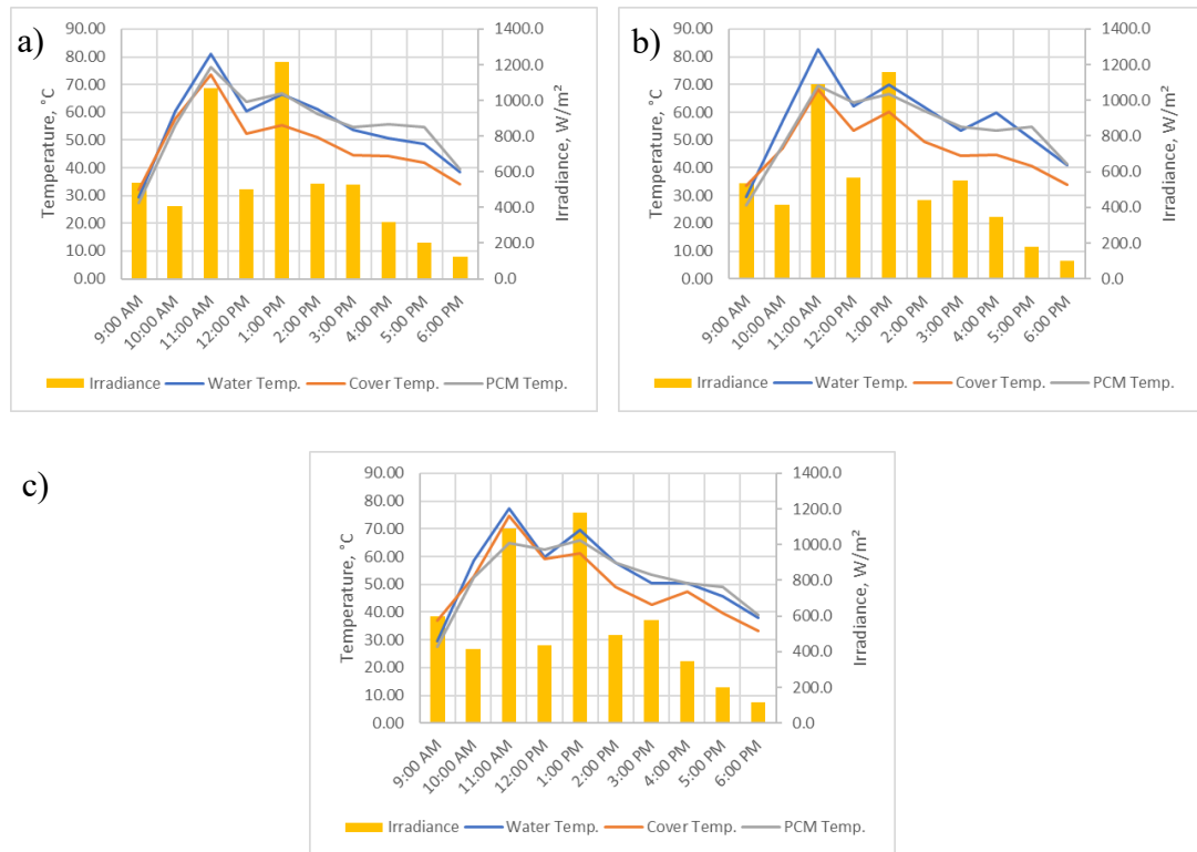
Figure 4.24: Temperature and irradiance results for different saline water using FL 33 cm Fresnel lens and Cu NPCM (a) 10k ppm (b) 20k ppm (c) 30k ppm
