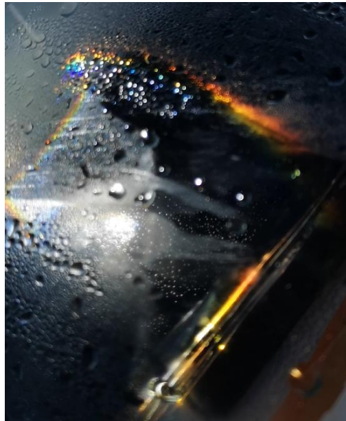
Figure 3.4: Aggressive bubble formation at the concentrated area under FL 33 cm Fresnel lens
