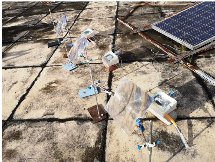
Figure 3.5: Outdoor experiment setup for comparing different saline water
