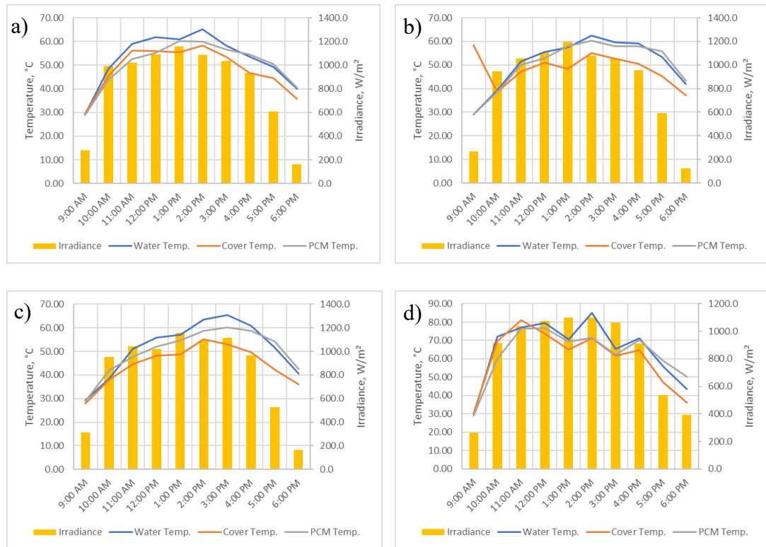
Figure 4.6: Temperature and irradiance results for different Fresnel lenses using 9k ppm saline water and Al scrap PCM (a) FL 12.7 cm (b) FL 9.9 cm (c) FL 20 cm (d) FL 33 cm
