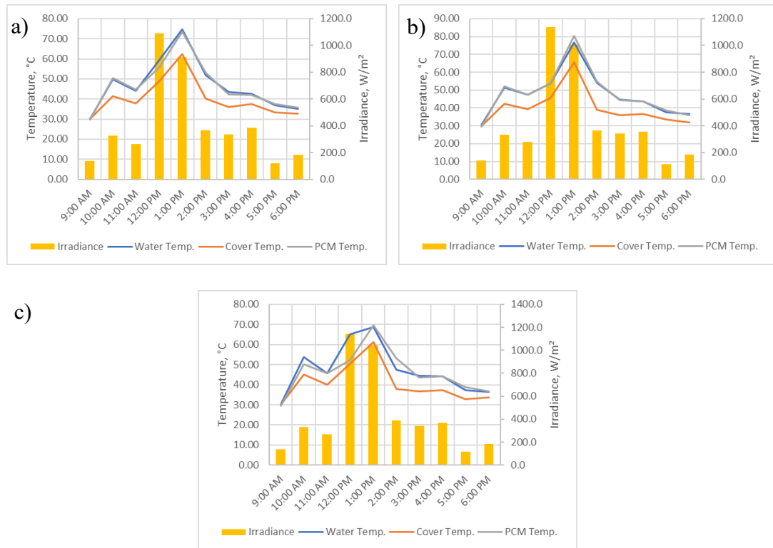
Figure 4.22: Temperature and irradiance results for different saline water using FL 33 cm Fresnel lens and Al 2 O 3 NPCM (a) 10k ppm (b) 20k ppm (c) 30k ppm
